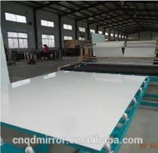
Film Covering Line (CAT I&II)
