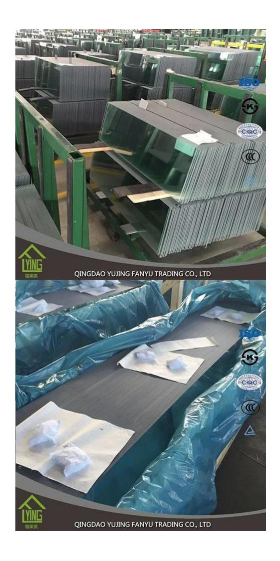
Tempered glass (toughened glass) 4-5 times stronger than annealed glass of equal thickness. Yujing tempered glass is a kind of safety glass that is very popular in building, decoration and automobile field. All work done on glass (beveling, cutting, bending, etc) must be done before tempering.
