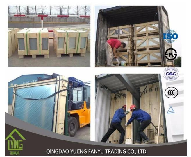
**Normal Packing**: Poly wood crate, cushion for shock absorption, plastic film for isolation of moisture, interlayer paper against scratch, metal staples for strengthening.
