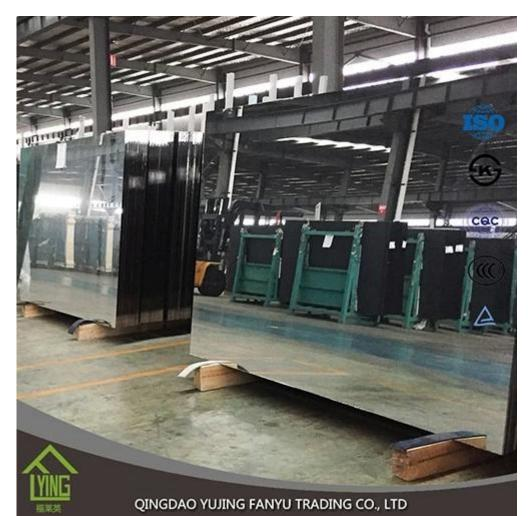
Yujing silver mirror is produced through a trine processing work by coating a silver film, a copper film, and two layers of waterproof paints on the surface of glass. Yujing have more than thirty sets of silver mirror and glass deep processing equipment, such as automatic cutting machine, milling machine, washing machine. Flat, round, oval, U shape, S shape mirrors are available, and round edge (also named as C-edge, pencil edge), flat edge, wave edge, beveled edge can be polished.
