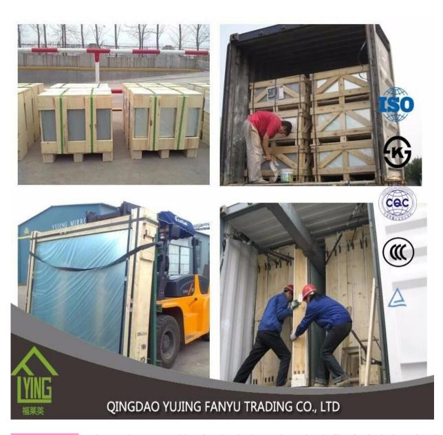
Normal Packing: Poly wood crate, cushion for shock absorption, plastic film for isolation of moisture, interlayer paper against scratch, metal staps for strenthening.
