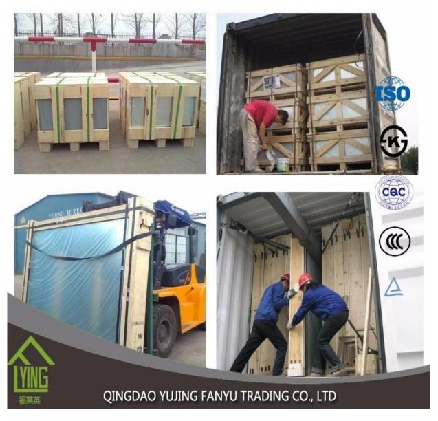
Normal Packing: Poly wood crate, cushion for shock absorption, plastic film for isolation of moisture, interlayer paper against scratch, metal staps for strenthening.
