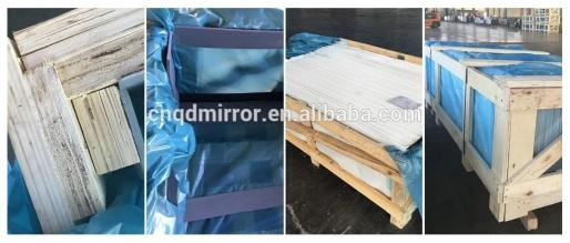
Packing: Standard seaworthy wooden crates with moisture-proof paper interleaved between two sheets
