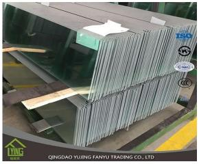
Fully tempered glass is 4-5 times stronger than annealed glass of equal thickness. All work done on glass(beveling, cutting, bending, etc) must be done before tempering.
