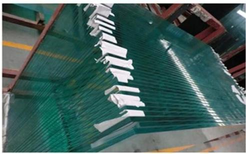
Yujing fully tempered glass 4 - 5 times stronger than annealed glass of equal thickness. All work done on glass (beveling, cutting, bening, ect) must be done before tempering. Tempered glass is one kind of high - strengh glass with even compressive stress on the srface hich is made by heaating float
