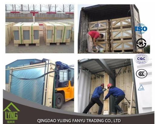
**Packing**Standard seaworthy wooden crates with moisture-proof paper interleaved between two sheets
